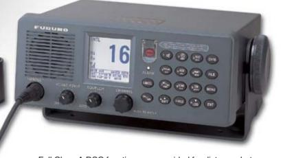
FURUNO FM-8800S/8800D are high quality, all-in-one marine VHF radiotelephones designed to comply with the GMDSS carriage requirements for safety and general communications. All the necessary functions such as a 25 W VHF radiotelephone, a Class A DSC modem and a CH 70 Watch Receiver are incorporated into the compact transceiver unit.
